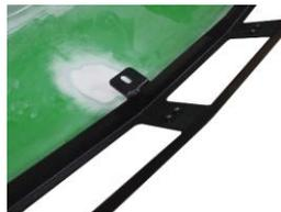
8. Polish the marked area on nose until it's white, and clean the surface, it should be no paint, dry and free of oil.
