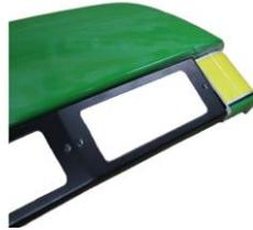
5. Check the installation of LED-4600 frame, it may take several times to align properly.
