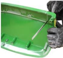
4. Use a hacksaw blade to cut the remaining corners, and polish the rough edges and corners.
