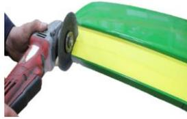
2. Cut the marks, in order to avoid the damage and reduce spintering, it would be better to use a cut-off wheel, rather than a Saw or Jigsaw, and cut it slowly.
