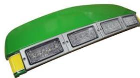
11. Install the LED lights in same direction to assure the wiring tabs are all facing the same way, mount front bezels using screws to hold lights in place, and tighten screws equally.
