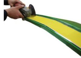
3. Measure 2" from the bottom of nose, and mark the line to cut, then make the cut on the underside of the marked line.
