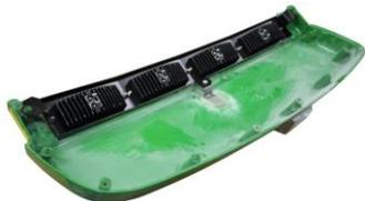
10. After 8~10 minutes, remove the LED-4600 frame, and reinstall nose to hood without frame. Once nose is installed on hood reinstall frame.
