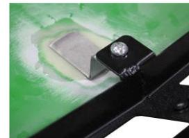
9. Mix the glue and spread thin layer at the marked area, install the tab according to slot on frame within 3~4 mins. And let's sit for 8~10 mins.
