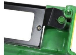
6. Check to make sure the slots on the tab are aligned with nose. And we may need to bend the tab a little.
