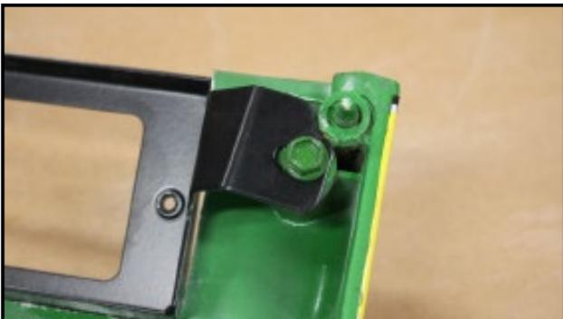
Check to make sure the new light housing bolt slot aligns with the nose. Tabs may have to be bent slightly to get correct alignment.
