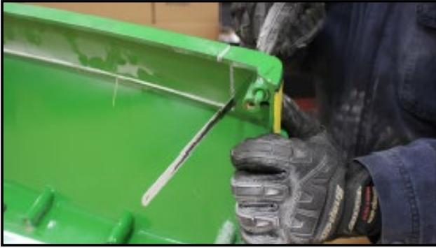
3. Next cut the remaining corners with hacksaw blade, and file the edges smooth.
