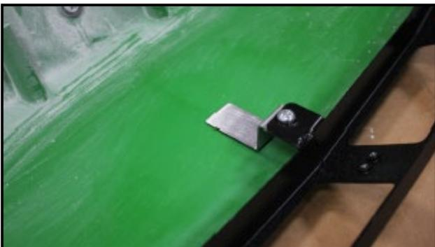
5. To install the Tab, bolt the light housing into the nose. Then, bolt the tab into the housing. Align the tab square with the housing, and make marks onto the nose outlining the tab.
