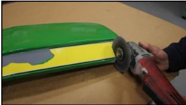
We used a right angle grinder with a 1/8" cutting blade to cut our marks. We didn't cut all the way to reduce splintering. Saw-zall or Jigsaws splinter fiberglass easily, so a cutoff wheel is preferred.
