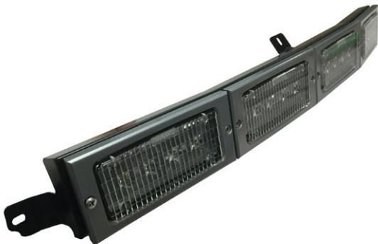
10. Since these tractors come with no lights form the factory, there is no wiring harness connection. You will have to find a wire from the switch or a fender light to connect to. Reinstall hood to tractor and bolt in place. Connect wiring and test lights.
